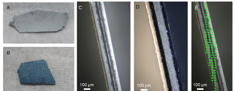
Figure 4: A, B) Photographs of two exemplary automotive paint samples c. c. D) Micrographs of the crosssections of the samples in A and B, respectively. E) Exemplary measurement grid (sample was measured with a tilt of eleven degree and the point distance was  $50 \mu\text{m}$ ).
