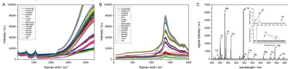
Figure 1: A, B) Raman spectra excited at A) 532 nm ( $I = 5 \cdot 10^4 \text{ W} \cdot \text{cm}^{-2}$ ,  $50 \times 1 \text{ s}$ ) and B) 785 nm ( $I = 2 \cdot 10^4 \text{ W} \cdot \text{cm}^{-2}$ ,  $50 \times 2 \text{ s}$ ) and C) LIBS spectra ( $5 \text{ mJ}$ ,  $10 \times 5$  pulses, delay:  $1.8 \mu\text{s}$ ) of the sixteen different glass samples.
