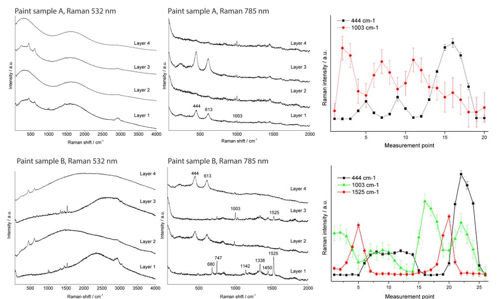
Figure 6: Exemplary Raman spectra obtained with excitation at 532 nm and 785 nm, respectively and the Raman intensity of selected bands in dependence of the measurement point.
