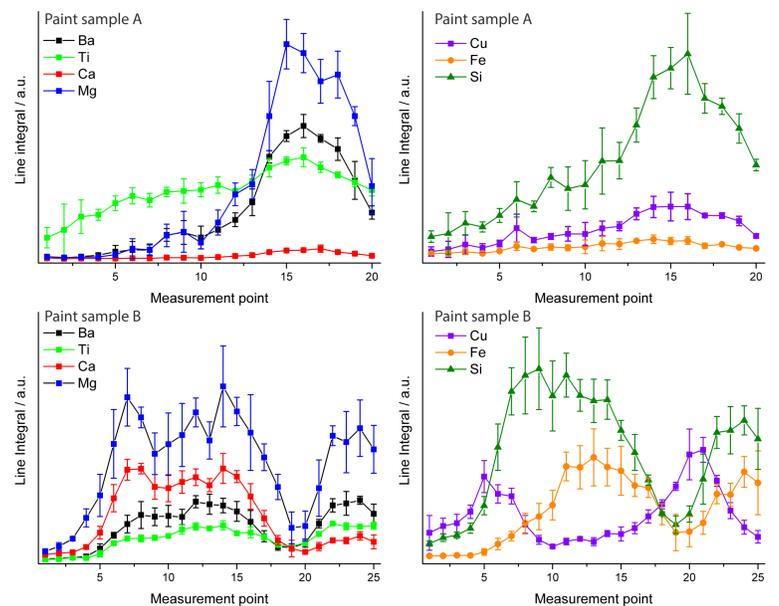
Figure 5: Distribution of line integrals of selected elements along the measurement points on the cross sections of the samples shown in Figure 4.
