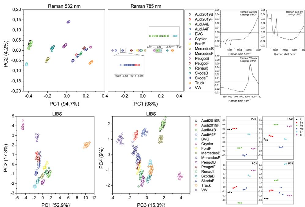
Figure 2: Scores and loadings resulting from the principal component analysis performed on the Raman spectra excited at 532 nm and 785 nm and the LIBS spectra, respectively.
